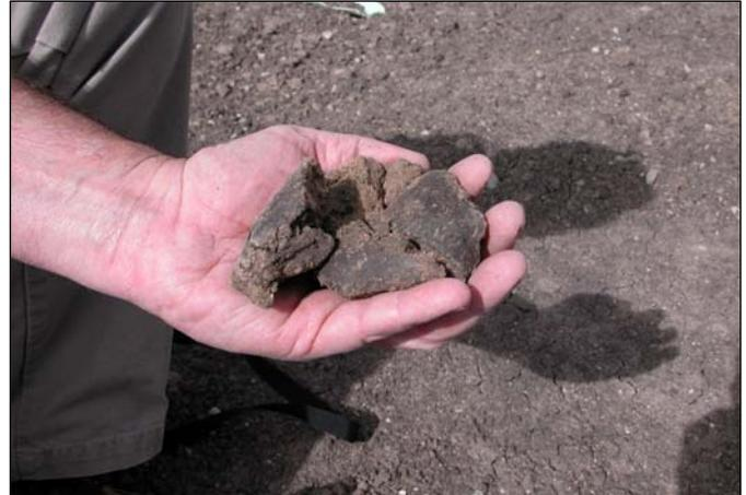
**Figure 2. Compaction of the Hollenbeck clay in the demonstration garden area of the Agricultural Center.**
