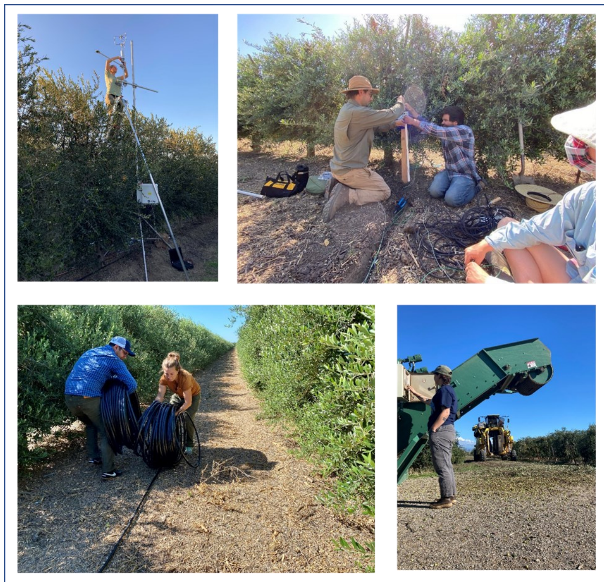
Figure 1. Installation of the ET station (top left), of soil moisture sensors (top right), of the irrigation system to apply the deficit (bottom left) and yield data collection (bottom right).
