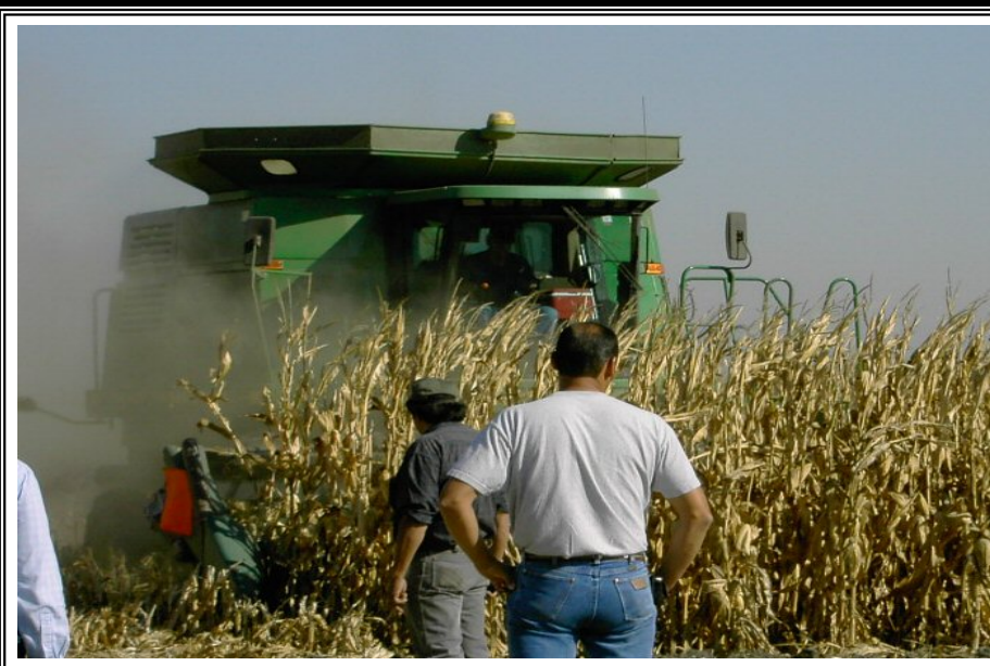
Some of the 120 participants at the San Joaquin Cooperative Extension 2005 Conservation Tillage Field Day watch the only combine in the state with a Geringhoff header mulch standing corn.
